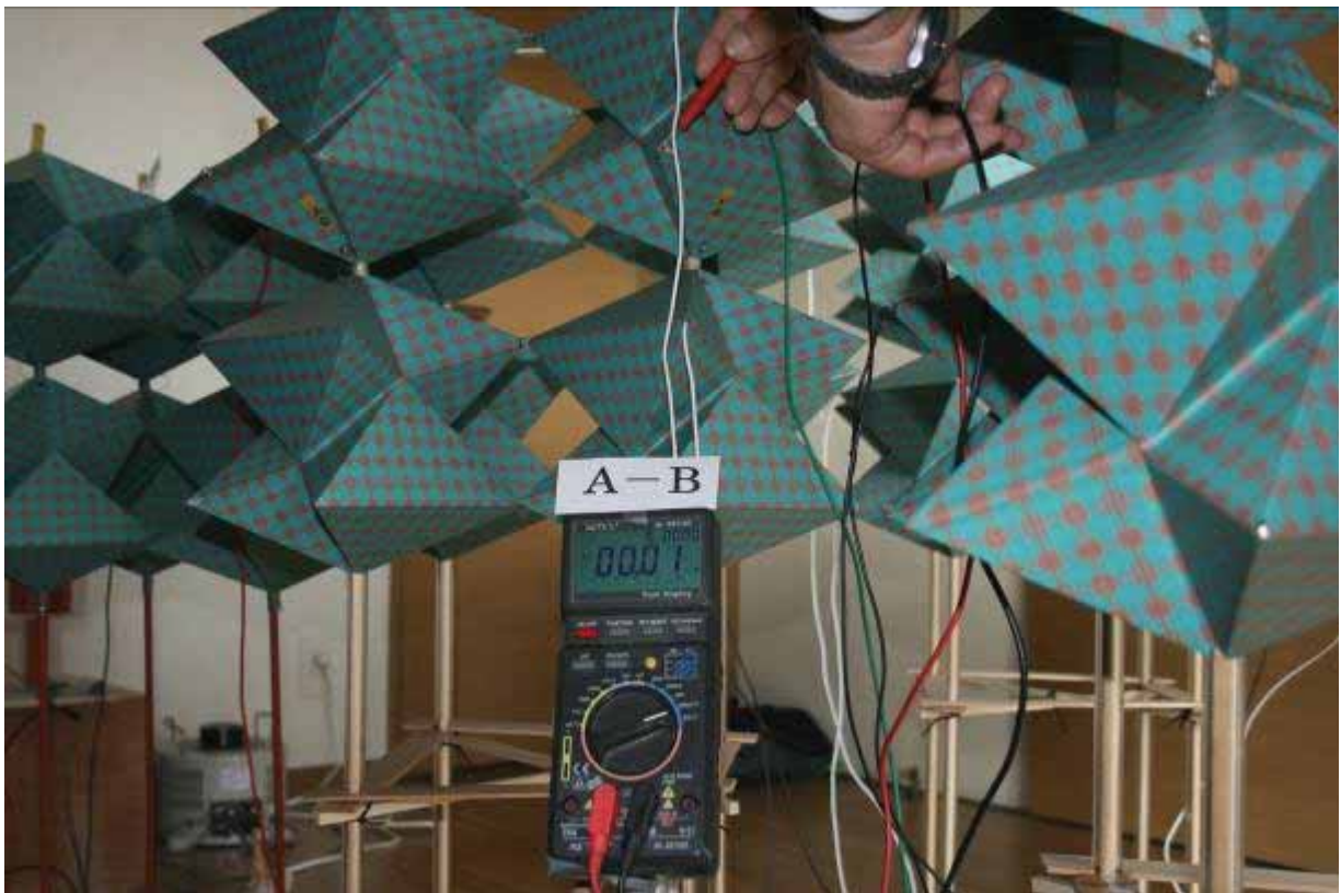
5 - 5 ' REAL CUBE "A" - REAL CUBE "B" (without power, with earth) AC 00.01 mA
